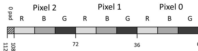
Figure 2-3: Three Pixels per Clock Format on s\_axis\_video\_tdata.
